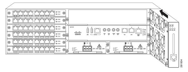
Step 2 Guide the fan tray into the chassis until it is fully seated.
